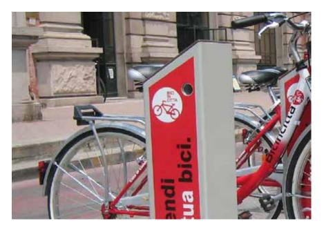
The display panels (approximately h2.5m x w1m) provide a point of visual reference for each station and offer graphic printed information for the users' reference. The absence of an electronic interface is a distinct advantage in many ways, since it reduces costs and complexity of the installation.
