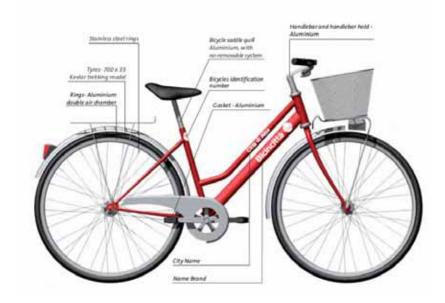
Although the bikes host a specification of robust components (metal pedals, hard-wearing tyres etc) it is not clear how many of the components are fastened with anything more secure than normal nuts and hex-head bolts. The seat post and quick-release adjustment for the seat are of a non-removable variety. Other specifications include dynamo driven lighting, v-brakes and a front basket for transporting users' belongings.
