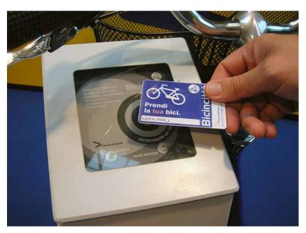
When new users register with the scheme, they are provided with a 'smart' proximity card, that uses RFID technology to store and transmit user details and the monitoring system connects these with the hired-
